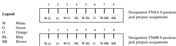
Eight-position jack pin assignments
